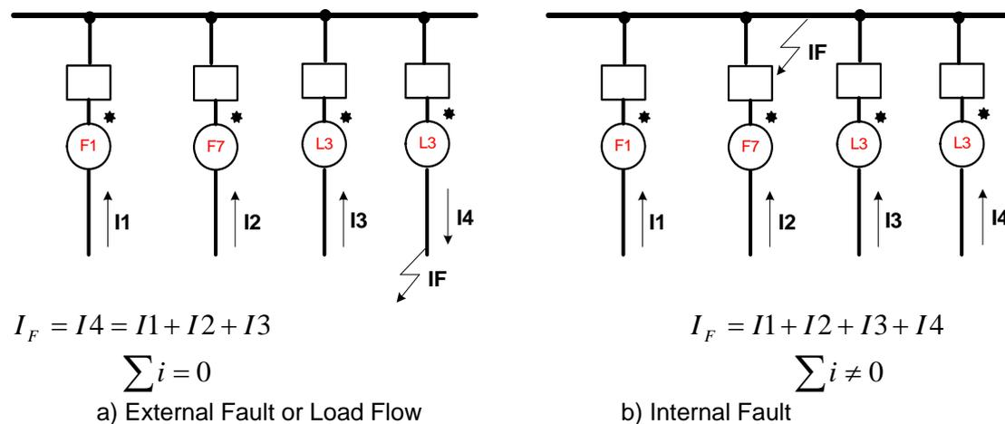
Figure 1: Bus Protection Operating Principle
