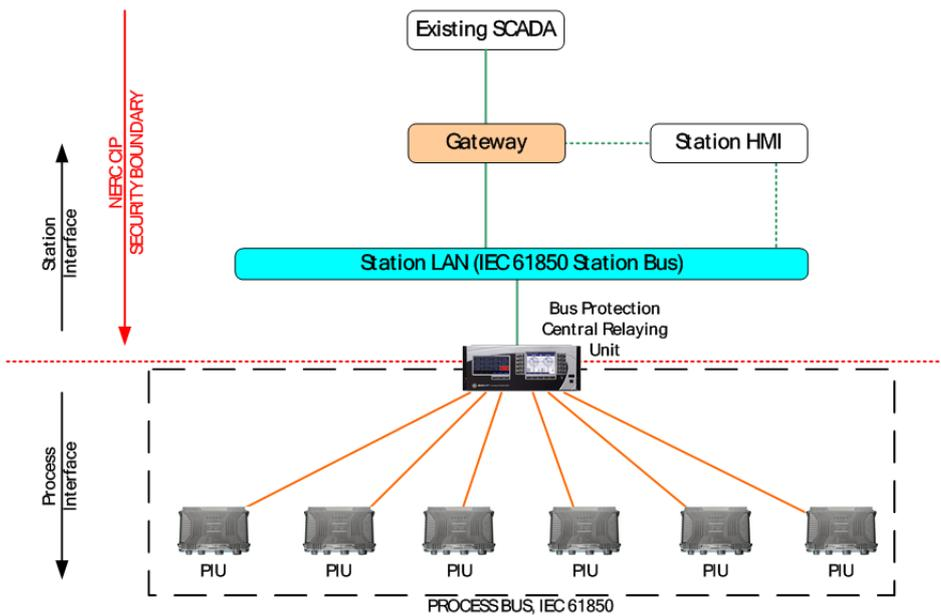
Figure 3: Natural Cyber-security Barrier
